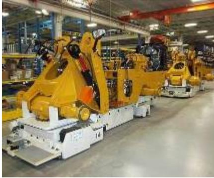
*Battery-free AGV in use at an off-highway vehicle assembly line. (RedViking - SAE technical paper 2014-01-0782)*
